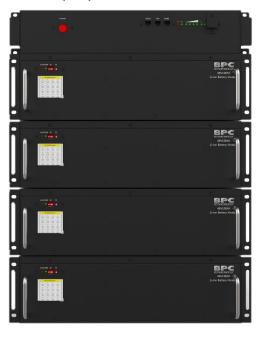
The larger BPC BCRT96VLFP options are designed to operate with the PowerGem Plus RT – LFP UPS 6kVA and 10kVA range and all operate from ±96 Volts nominal battery voltage with options for 12Ah, 50Ah and 100Ah.
