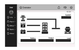
Colour 7 inch touch screen LCD display panel providing all UPS control parameters, status and alarm information.
