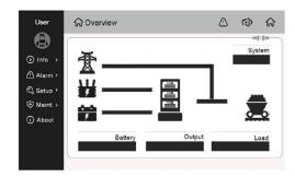
Colour 7 inch touch screen LCD display panel providing all UPS control parameters, status and alarm information
